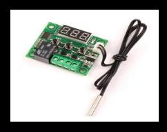
© TEMPERATURE SENSOR IS USED TO MEASURE THE TEMPERATURE TO MAINTAIN CONSTANT TEMPERATURE INSIDE THE VESSEL
