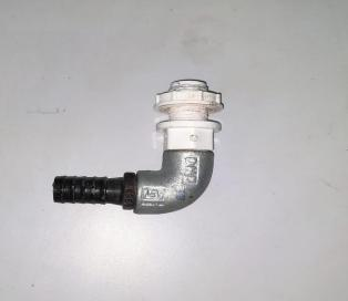
© OUTLET PIPE IS PLACED IN THE BOTTOM OF THE XL VESSEL TO REMOVE THE WATER FROM THE VESSEL
